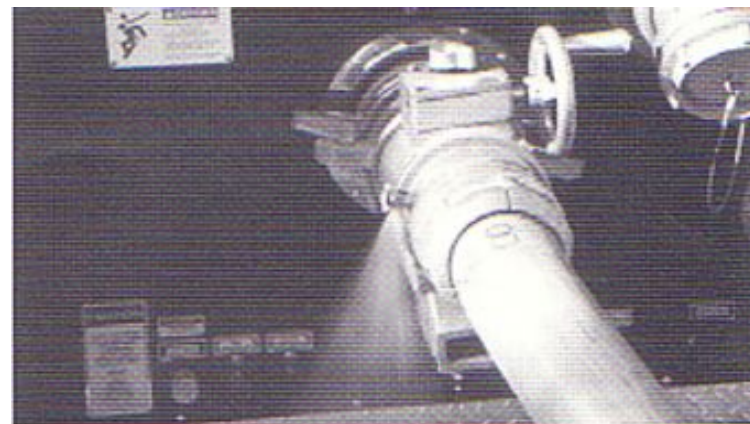
Figure 13.7 Use the bleeder to discharge air from the hose as it is charged with water.
